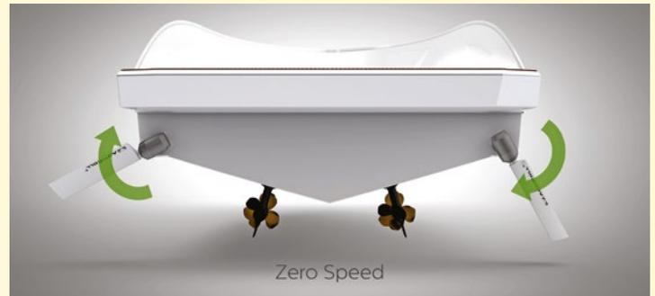
Dynamic Marine Systems (DMS) Holland, who successfully developed and launched the MagnusMaster, has now started developing a new product. Thanks to MagnusMaster's success and a grant, DMS Holland, along with Brabant Engineering, is developing a roll damping system for fast-planing yachts up to 30 meters called AntiRoll, a damping system that will be produced as a standard-series stabilizer.
