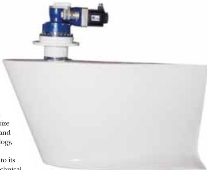
CMC'S STABILIS ELECTRA S.E. FIN & ACTUATOR DESIGN.
